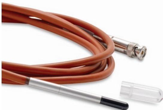
The 0.3 cc ionization chamber is designed for measurements in the useful beam of high-energy photon and electron fields. The waterproof chamber is used mainly for relative measurements in a water phantom or air scanner. The measuring volume is open to the surrounding air via the 1.3 m (4.3 ft) cable and BNC Triax connector. This chamber has a short and rigid stem for easy mounting, includes a PMMA buildup cap, and is type tested by PTB Braunschweig.
