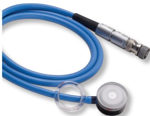
The Markus chamber is the very first chamber specifically designed for electron dosimetry. The chamber may be used for measurements in water phantoms or solid-state phantoms. A PMMA waterproofing cap, 0.87 mm thick (equivalent to 1 mm of water), and an annulus for solid-state phantom measurements are included. The chamber's small measuring volume makes it ideal for electron measurements when very high spatial resolution is required. The diaphragm front
