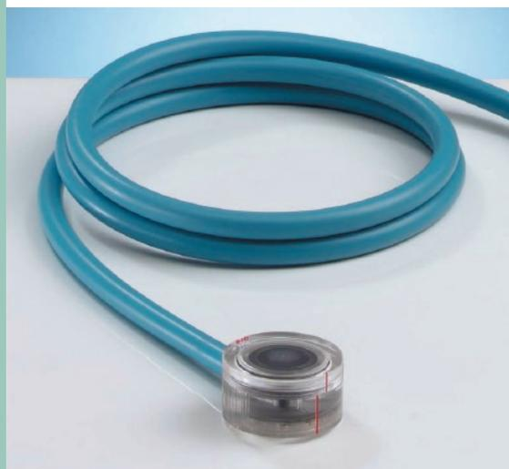
The 0.02 cc Advanced Markus Chamber is our newest development in plane-parallel electron ion chambers. This chamber combines the advantages of both Roos™ and Markus chamber types into one truly exceptional plane-parallel electron chamber. Developed for relative and absolute electron dosimetry in water or solid type phantoms, the advanced design of this chamber makes it possible to perform absolute electron dosimetry without perturbation effects.
