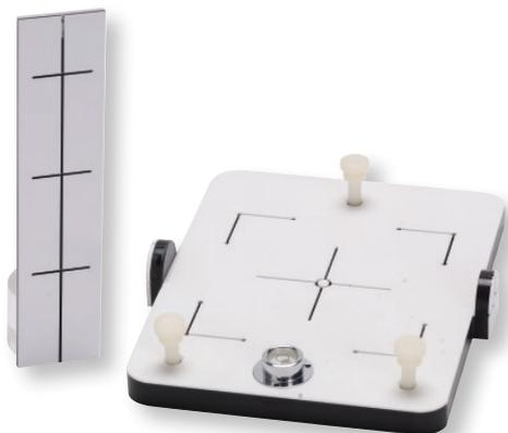
Accuracy begins with beam alignment. It is impossible to deliver the carefully-calculated plan if the beam position is not verified. TEL-ALIGN verifies the coincidence of the light and radiation fields and checks the isocenter variation and the optical back pointer when the gantry is rotated  $\pm 90^\circ$ .
