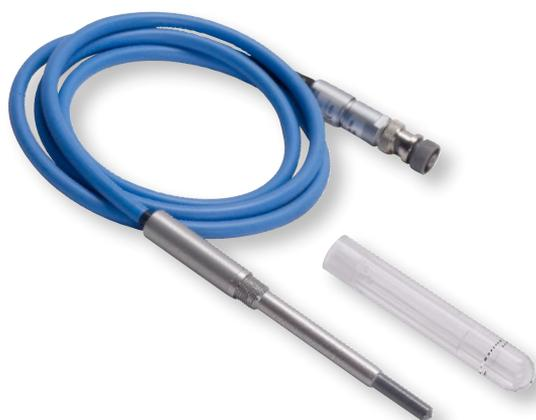
The waterproof 0.6 cc ionization chamber is designed for absolute dosimetry in radiation therapy. Since the chamber is waterproof, it may be used in water phantoms and does not require a protective sleeve. It is rugged in construction and has a PMMA/graphite thimble and an aluminum electrode. This chamber includes a 1 m (3.3 ft) cable, BNC Triax connector, and a PMMA buildup cap.
