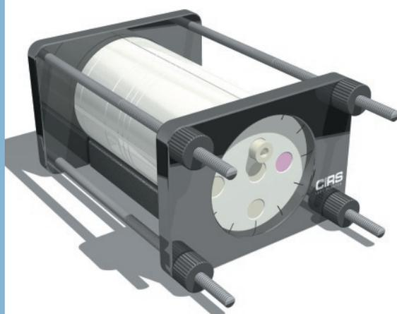
The 74-001 IMRT phantom is designed to address the complex issues surrounding commissioning and comparison of treatment planning systems and verification of individual patient plans and delivery.
