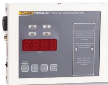
The PRIMALERT Digital Area Monitors are designed for a wide range of gamma radiation area monitoring applications. Two self-contained configurations are available, each with an internal energy compensated GM detector (detection range in parentheses): 05-443 (0.1 mR/h to 1 R/h) and 05-444 (1 mR/h to 4 R/h). Both models are ac powered with an internal battery backup, have user-settable low and high alarms, and are available with an optional remote alarm for added security.
