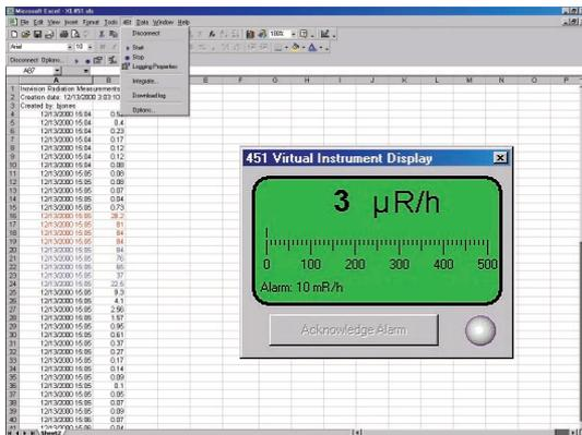
The 451EXL provides remote control for many of the 451B and 451P functions via a Microsoft® Excel-based user interface, including real-time data logging with user-defined alarm parameters, upload of the internal data log into Excel worksheet, real-time virtual instrument display, and accumulated dose measurement over a user-defined integration period. This information management software is ideal
