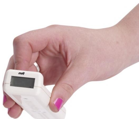
The slim, compact Beeper mR is the ideal personal monitoring device for alerting personnel to the presence of radiation in medical, industrial or research settings. It accurately measures and displays the radiation dose received.
