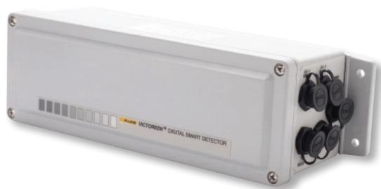
The versatile 1060AM is designed for reliable, continuous area monitoring for gamma or x-ray sources in a medical facilities, or any other facility with radioisotope sources. Employing internal Geiger-Mueller (GM) detectors, it is available in environmental, low, medium, and high range versions, with an optional MHV interface that can accommodate a wide variety of external GM probes.
