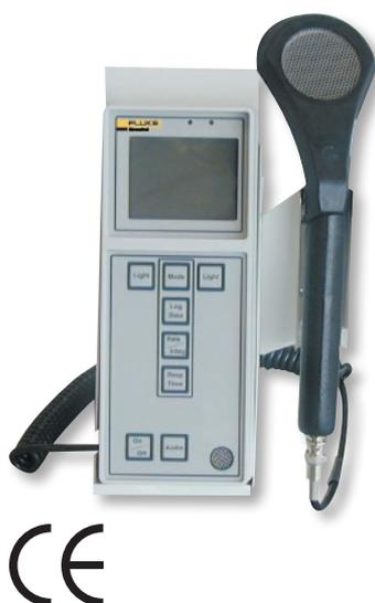
The easy-to-use, auto-ranging 190F is compatible with GM detectors, neutron probes, proportional counters, and scintillation probes operating from 300 volts to 1,300 volts. Depending on probe selection, the 190F detects alpha, beta, gamma, x-ray or neutron radiation within an operating range of 1  $\mu\text{R/h}$  to 1 R/h (1 CPM to 1,000,000 CPM). The unit is available with either an MHV or a BNC connector.
