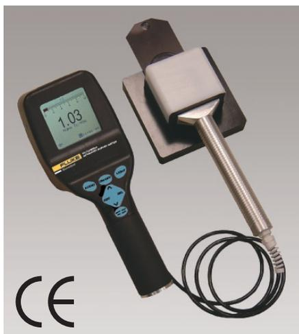
The Wipe Test Fixture for Advanced Survey Meter (Model 489-200WTF) uses a high efficiency NaI(Tl) scintillation probe (Model 489-200) in conjunction with a lead-shielded sample holder. It employs a removable wipe-test holder or tray positioned below the shielded probe. Under these conditions, background radiation is minimized and wipe-test counting is maximized.
