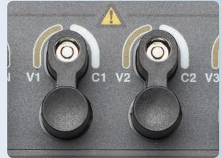
Insulated applied parts connections
