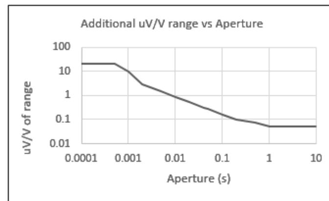
Aperture  $\geq 100 \mu\text{s}$ ; additional uncertainty with read rate: (Read Period = aperture + delay between readings)
