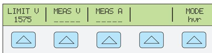
With the Calibrator in Operate mode, the resistance across the MEGOHM terminals can be changed through the keypad or the rotary knob.
