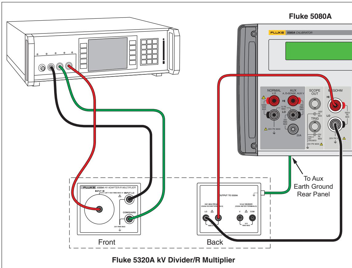
Figure 9. Connections to Bench Tester with a Resistance Multiplier Adapter
