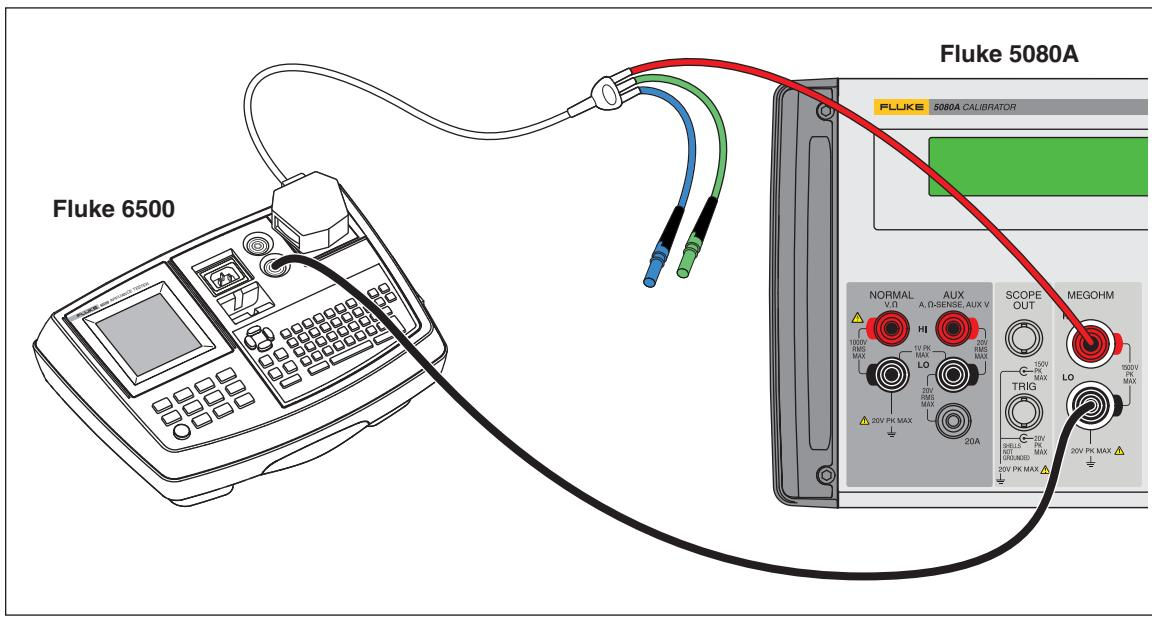
Figure 6. Calibrating Insulation Resistance of a Portable Tester
