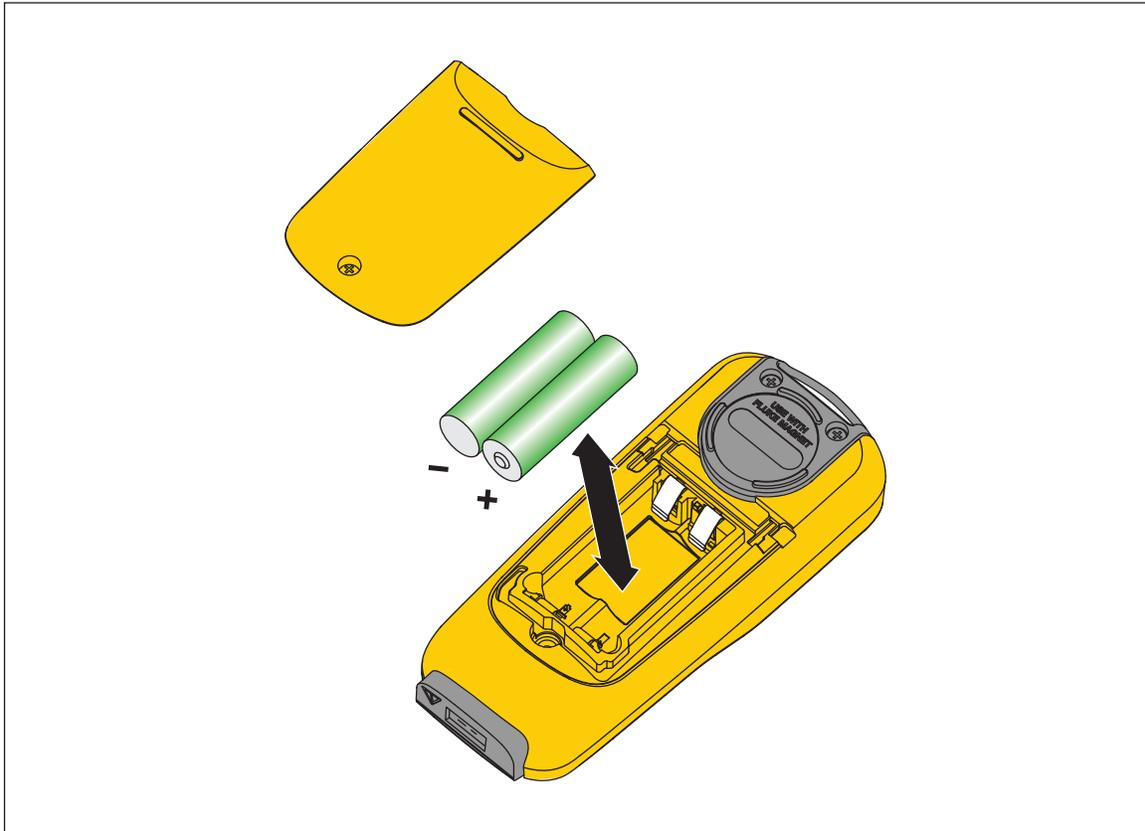
**Figure 4. Battery Replacement**
