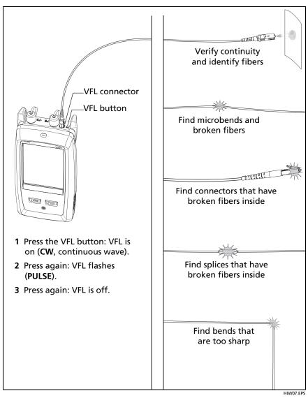
Figure 26. How to Use the Visual Fault Locator
