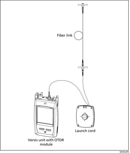
Figure 13. OTDR Connected with a Launch Cord
