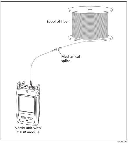
Figure 15. OTDR Connected to a Spool of Fiber
