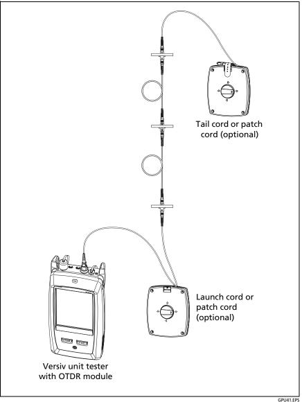
Figure 21. FaultMap Test Connections
