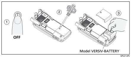
Figure 33. How to Remove the Battery
