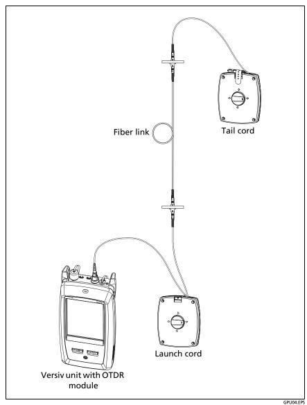
Figure 14. OTDR Connected with Launch and Tail Cords
