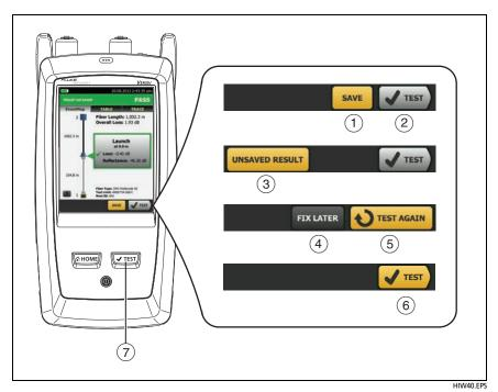
Figure 4. FIX LATER, TEST AGAIN, and TEST Buttons and the TEST Key
