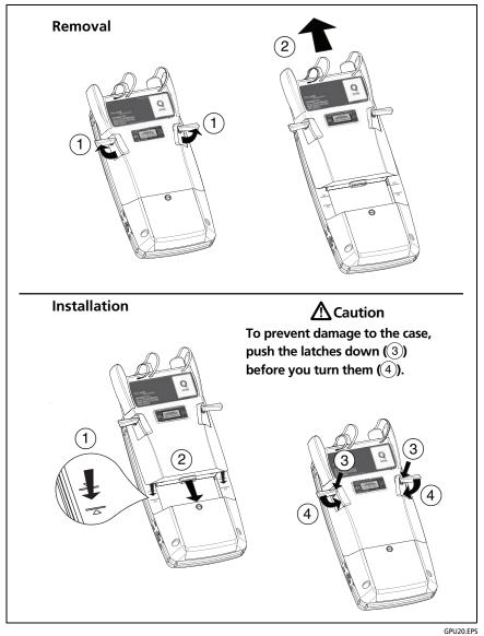
Figure 6. How to Remove and Install the Module
