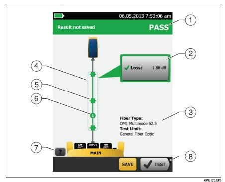
Figure 25. Result for Far End Source Mode
