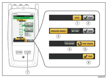
Figure 7. FIX LATER, TEST AGAIN, and TEST Buttons and the TEST Key
