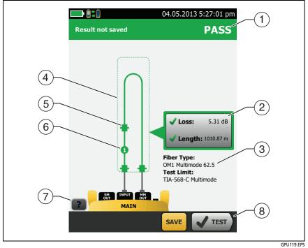
Figure 22. Result for Loopback Mode
