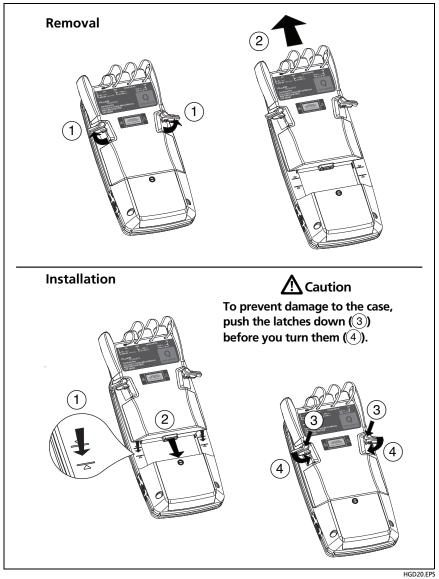
Figure 10. How to Remove and Install a Module
