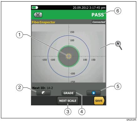
Figure 27. FiberInspector Image with Measurement Scales (fiber with 50 µm core shown)
