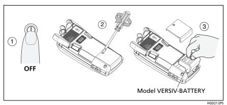
Figure 40. How to Remove the Battery
