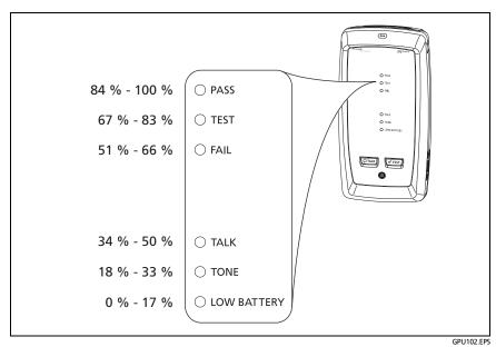
Figure 4. LEDs Show the Remote's Battery Status
