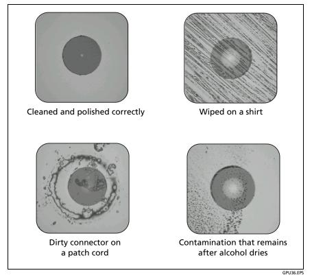
Figure 11. Examples of Clean and Dirty Fiber Endfaces
