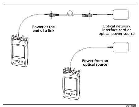
Figure 31. Connections to Monitor Power and Loss
