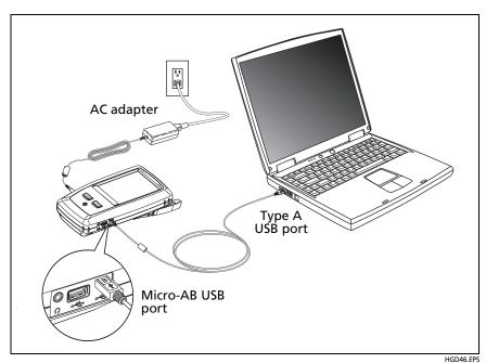
Figure 35. How to Connect the Tester to a PC
