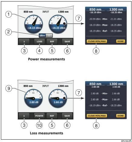
Figure 32. Power Meter Measurements and Controls
