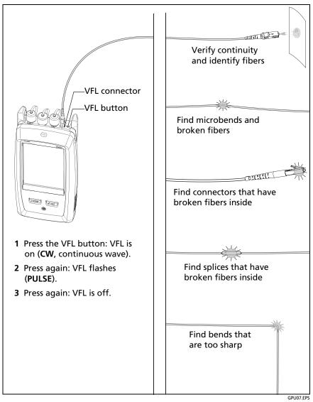
Figure 29. How to Use the Visual Fault Locator
