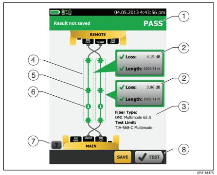
Figure 19. Result for Smart Remote Mode (Unsaved Bi-Directional Results Shown)
