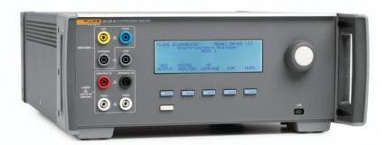
The QA-ES III Electrosurgical Analyzer simplifies testing to ensure the performance and safety of electrosurgical units. With generator output current accuracy as low as  $\pm$  2.5 %, the QA-ES III is capable of testing all modern high power electrosurgical units.
