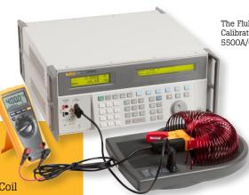
The Fluke 5500E Multi-Product Calibrator and the optional 5500A/COIL 50 turn current coil.
