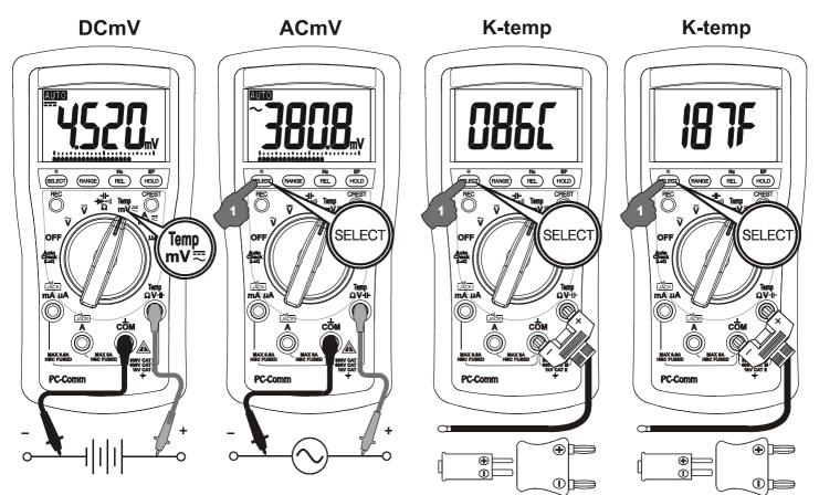
Note: Be sure to insert the banana plug K-type temperature bead probe Bkp60 with correct polarities. You can also use a plug adapter Bkb32 (Optional purchase) with banana pins to K-type socket to adapt other standard K type mini plug temperature probes.
