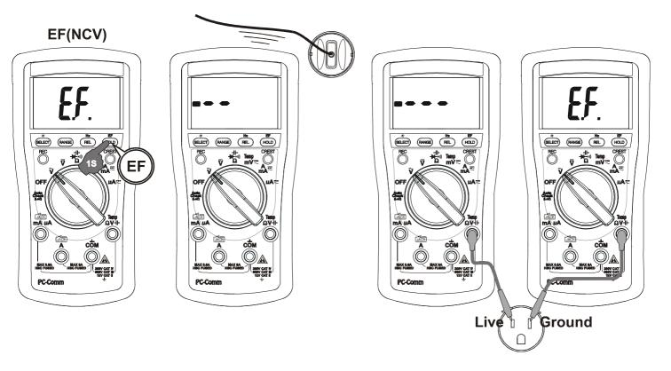
•**Non-Contact EF-Detection:** An antenna is located along the top-right end of the meter, which detects electric field surrounds current-carrying conductors. It is ideal for tracing live wiring connections, locating wiring breakage and to distinguish between live or earth connections.
