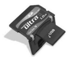
To change the card function to USB, hold the card with the label upwards, and hinge the outer section of the lower half of the card downwards. This exposes a USB connector which can be plugged into a standard USB port on a computer.
