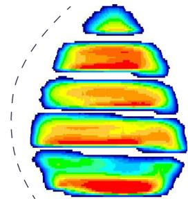
Same Tire in a 3.5° Slip Angle Test, Captured at 48 km/h (30 mph)
