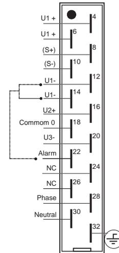
Figure 2. Pin-out 2 to 3 output with Connector DIN41612, H15
