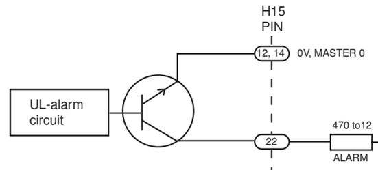
Figure 5. Open collector alarm and inhibit input.
