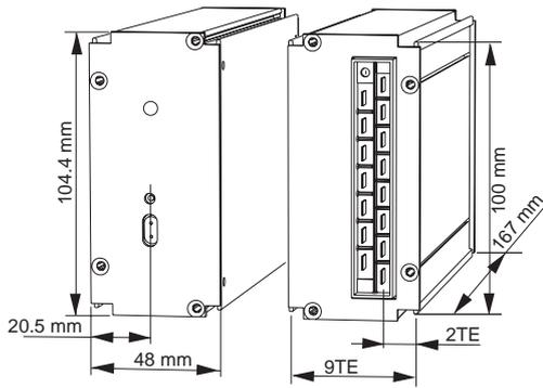
Figure 7. Front and connector side of PSC100
