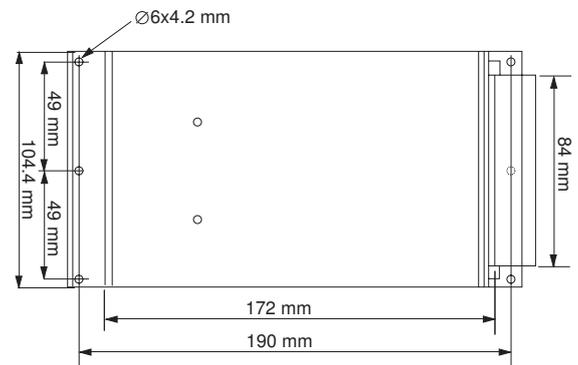
Figure 11. Top view on wall mounting option N
