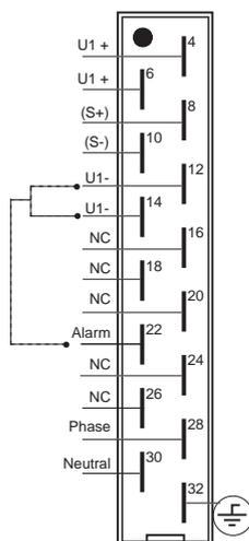
Figure 1. Pin-out single output with Connector DIN41612, H15.
