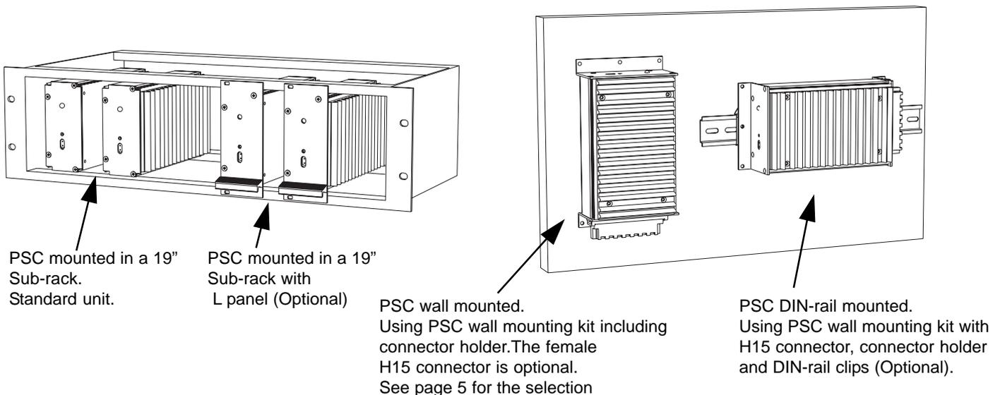
PSC mounted in a 19" Sub-rack. Standard unit.
