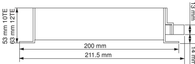
Figure 10. Side view on wall mounting option N
