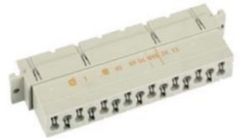
Figure 5. H15 Cage Clamp type female - H15-CC The cable rating is AWG16 or <1.5 \text{ mm}^2 . That makes it not usable for 24T-input and 5 V outputs.
