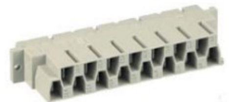
Figure 6. H15 FastOn 6.3 mm female - H15-T The TABS are rated 12 A 70°C or 15 A 55°C thus 2.5 \text{ mm}^2 or AWG13
