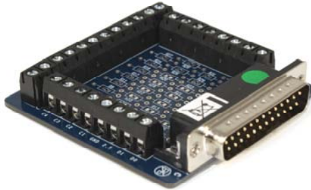
Figure 1 - Small Terminal Board
