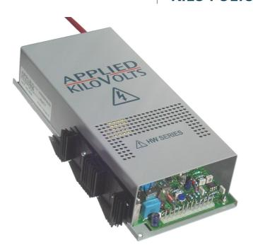
The HW series of high voltage modules covers the range from 1kV to 50kV giving 100Watts of output power. Control of the output voltage is by internal potentiometer or by external potentiometer or by an external 10 volt analogue control voltage. Pins 1 to 10 of the 12 pin Molex input connector are pin compatible with both the high precision HP series and the general purpose KS series (please see separate data sheets).
