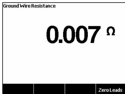
Figure 10. DUT Ground Resistance Measurement
