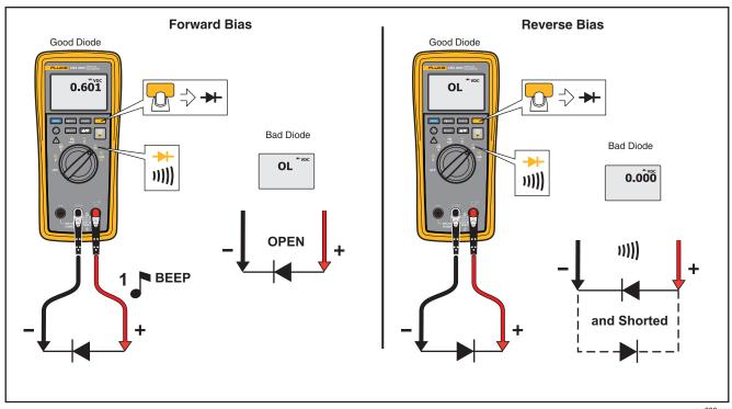
Figure 7. Diode Test
