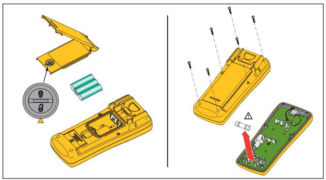
Figure 11. Battery and Fuse Replacement
