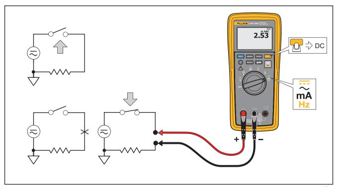
Figure 6. AC and DC Current Measurements
