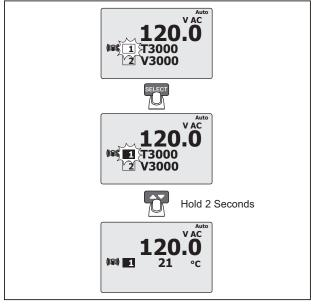
Figure 9. Module Binding Procedure
