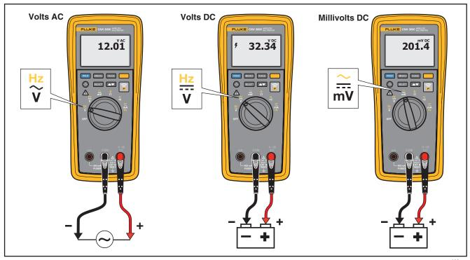
Figure 1. AC and DC Voltage Measurements
