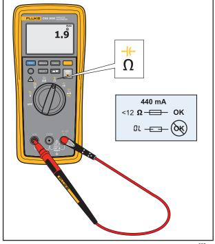
Figure 10. Fuse Test
