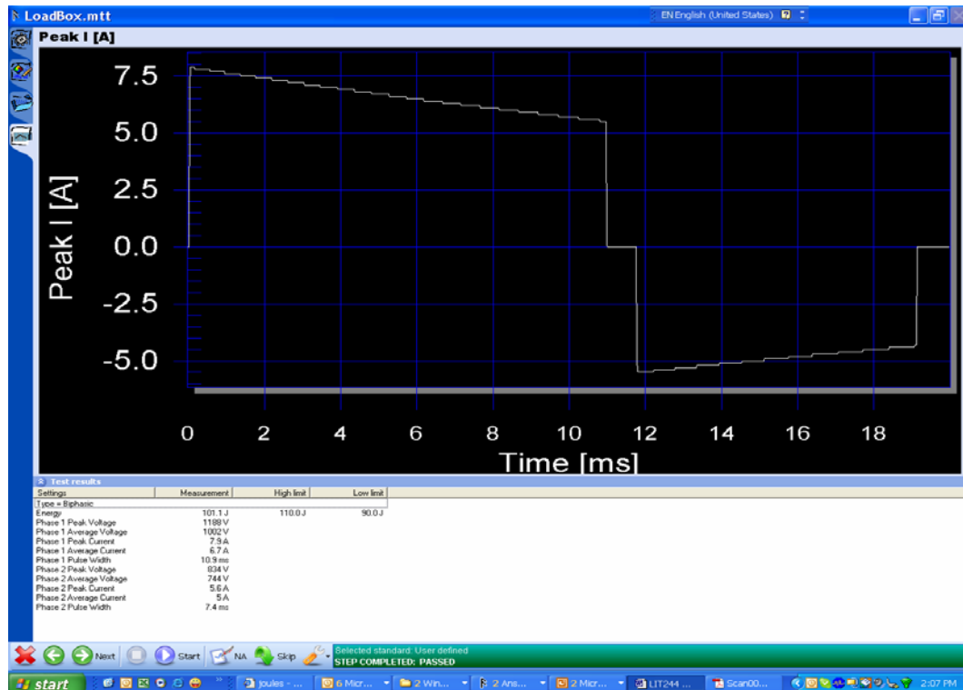
Figure 2: defibrillator discharge curve during energy measurement test (external load 150 ohms, preset energy level 100J)
