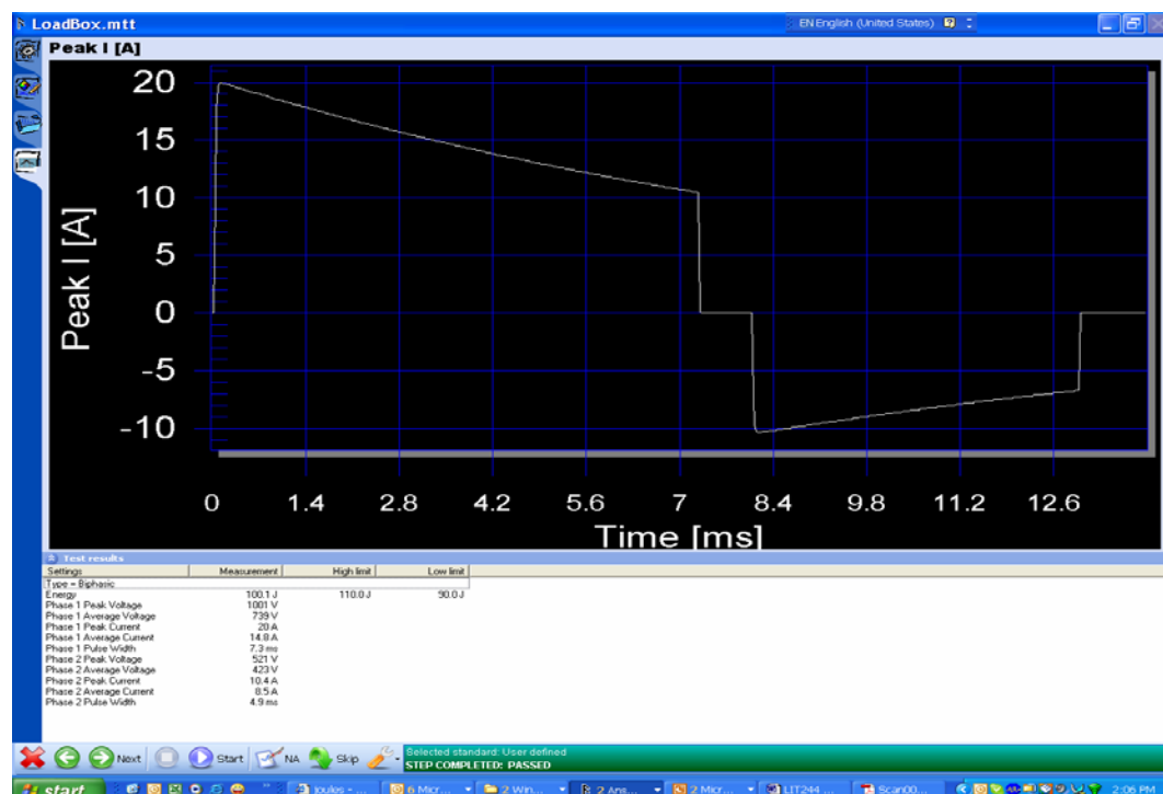
Figure 1: defibrillator discharge curve during energy measurement test (external load 50 ohms, preset energy level 100J)
