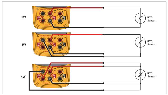
Figure 7. Measure Temperature with an RTD
