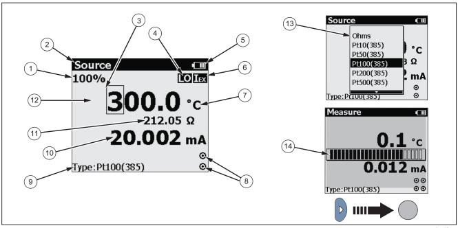
Figure 4. Elements of a Typical Display
