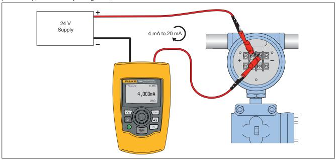
Figure 20. In Circuit, External Loop Power Connections
