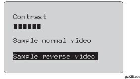
Figure 16. Contrast Adjustment Screen
