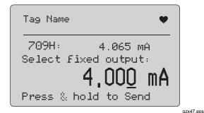
Figure 38. Set Fixed mA Output Screen
