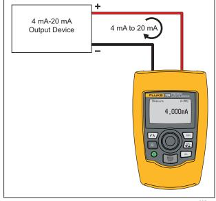
Figure 6. mA Measure Connections
