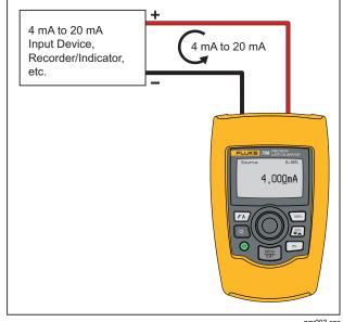
Figure 4. mA Source Connections
