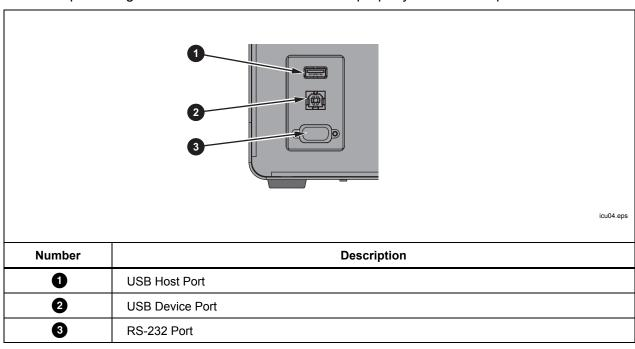
Figure 14. Remote Interface Ports
