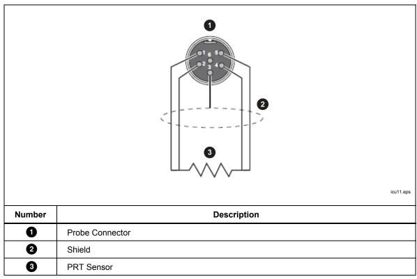
**Figure 11. Reference Probe Connections**
