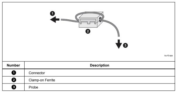
Figure 10. Ferrite Installation
