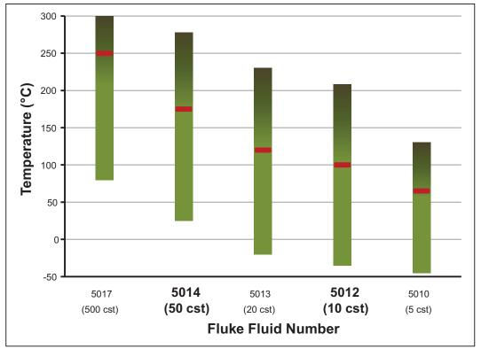
Figure 15. Silicone Fluid Temperature Ranges
