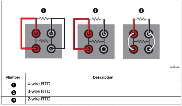
Figure 12. Test RTD Connections
