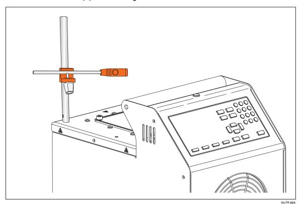
Figure 8. Probe Clamp Accessory
