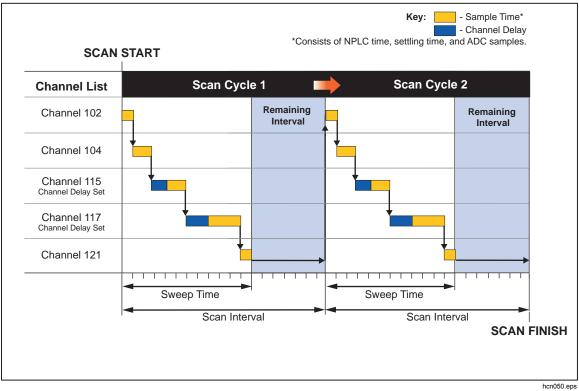
Figure 4-2. Illustration of a Scan Sweep
