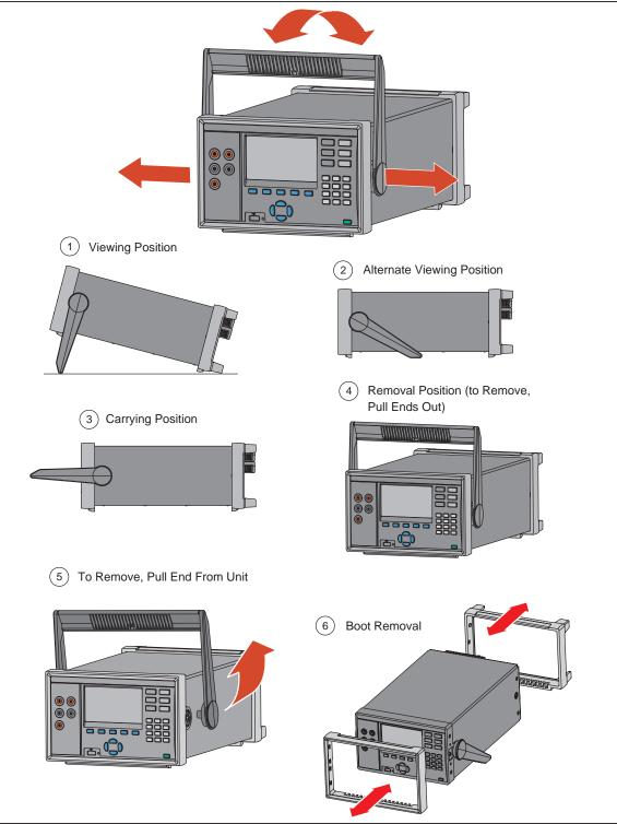
Figure 2-3. Handle Positions and Boot Removal
