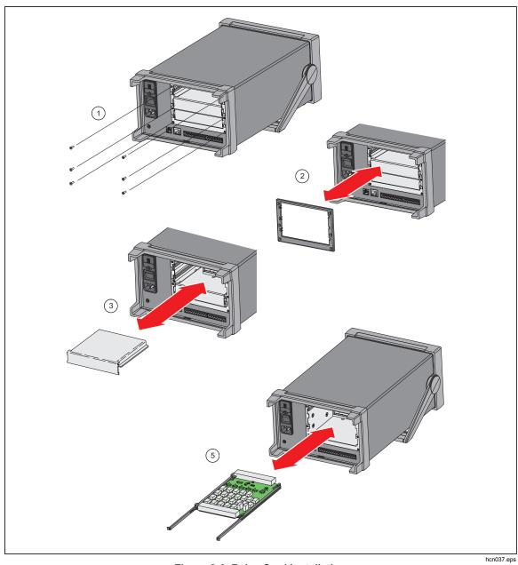
Figure 2-6. Relay Card Installation
