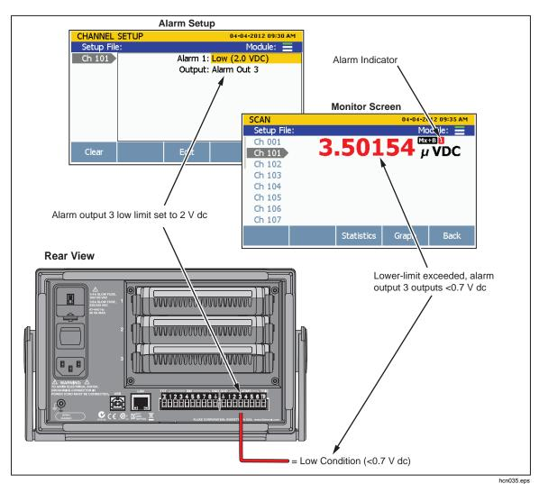
Figure 3-10. Alarm Output Example
