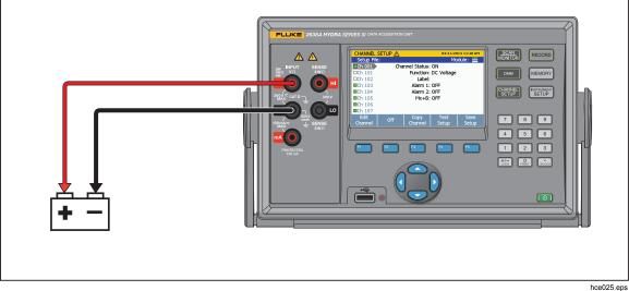
Figure 5-1. Example Voltage Front-Panel Connection
