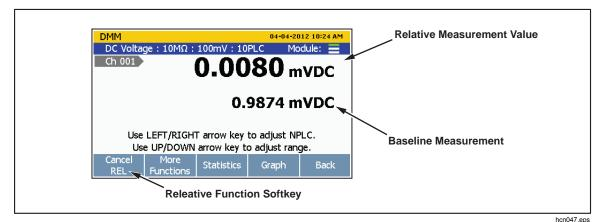
5. Observe subsequent readings as relative measurements.
