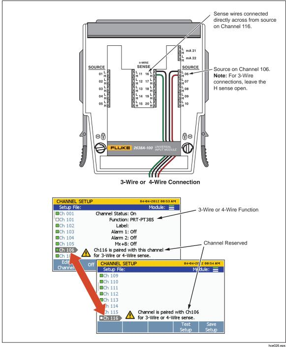
Figure 3-2. 3-Wire and 4-Wire Channel Reservation
