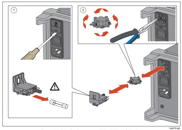
Figure 2-1. Fuse Replacement and Line-Voltage Selection
