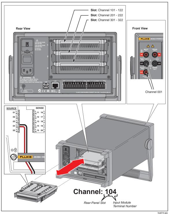
Figure 3-4. Example Channel Assignment
