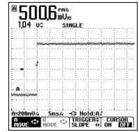
Figure 2-13. Making a Single Acquisition
