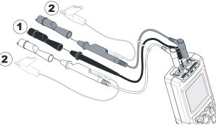
Figure 2-3. Volts Measurement Setup
