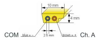
As-i also uses M12-connectors for data as well as on/off signals. The figure below shows where to find + and - on on such a connector.
