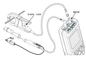
Figure 3-1. Input Connections for Harmonics
