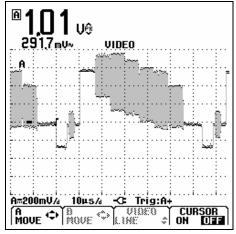
Figure 2-17. Measuring Video Signals
