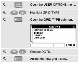
Use LINES when you need a cross hatch pattern based on the horizontal time and vertical divisions on the screen. Use DOTS when you need vertical and horizontal division dots as added reference points to the screen.
