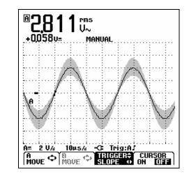
Figure 2-12. Displaying the Envelope of a Waveform
