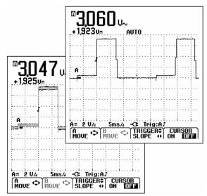
Figure 2-11. Smoothing the Waveform
