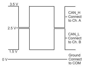
To check CAN Bus, ScopeMeter Channel A and B are on and DC coupled. The recommended probes are STL120 (1:1). Probe Tip A must be connected to CAN\_H, B to CAN\_L, and COM to CAN\_GND.
