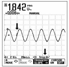
Figure 2-15. Screen with all Trigger Information
