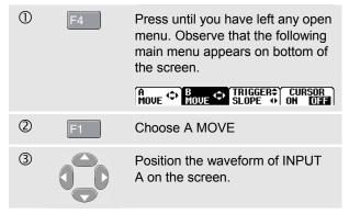
Waveform positioning is demonstrated in Figure 2-10.
