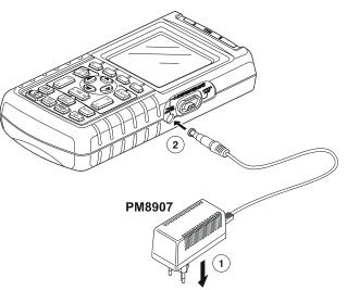
Figure 8-1. Charging the Battery Pack
