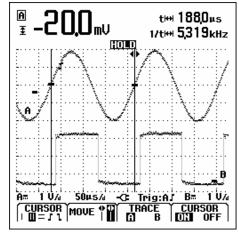
Figure 2-19. Time Measurement with Cursors
