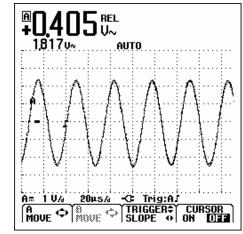
Figure 2-9. Making a Relative Measurement
