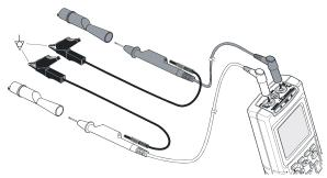
Figure 9-2. Grounding with Short Ground Lead
