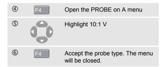
Observe that the 10 times attenuation of the Probe is compensated in the voltage readout.
