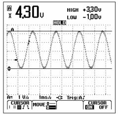
Figure 2-18. Voltage Measurement with Cursors
