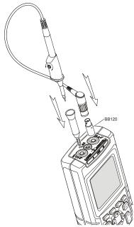
Figure 8-3. Adjusting Scope Probes
