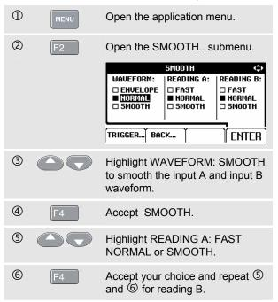
WAVEFORM SMOOTH suppresses noise without loss of bandwidth. Waveform samples with and without smoothing are shown in Figure 2-11.
