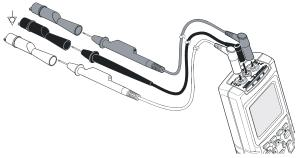
Figure 9-3. Grounding with Unshielded Ground Lead
