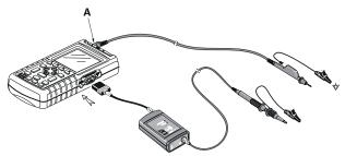
Figure 2-16. Isolated Triggering
