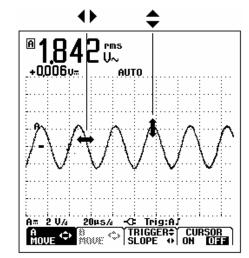
Figure 2-10. Positioning the Waveform
