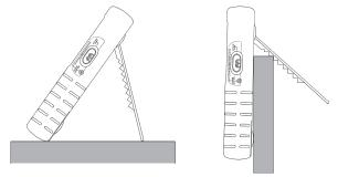
Figure 9-1. Using the Tilt Stand
