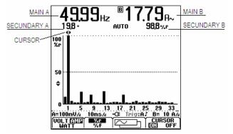
Figure 3-3. Reading the Harmonics Screen
