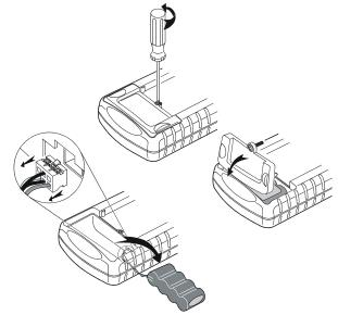
Figure 8-2. Replacing the Battery Pack
