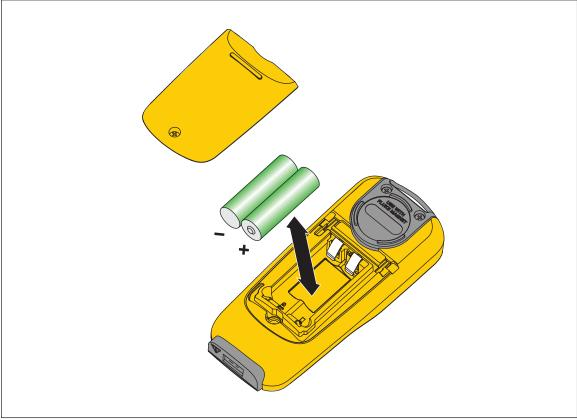
Figure 4. Battery Replacement
