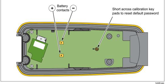
Figure 3. Calibration Password Reset
