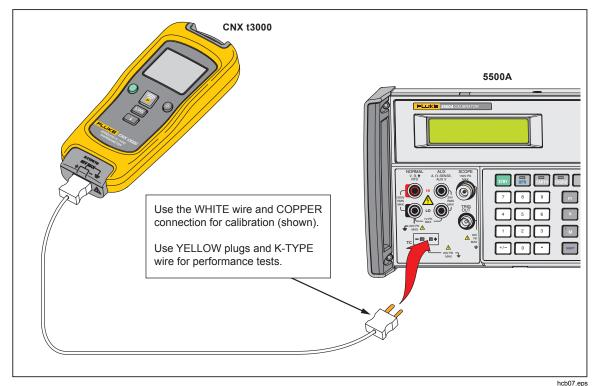
Figure 2. Performance Test and Calibration Connections
