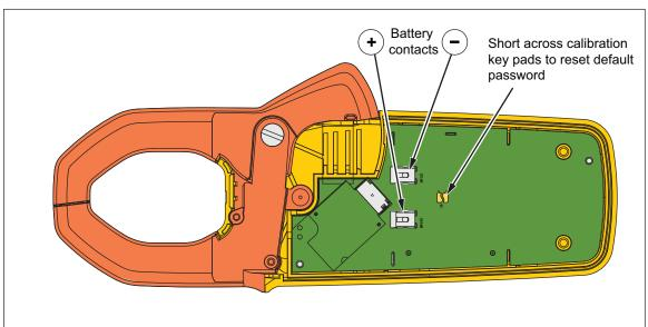
Figure 4. Calibration Password Reset
