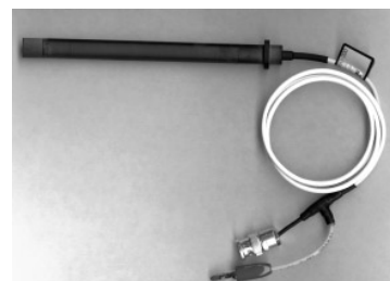
10 cc high sensitivity ion chamber
