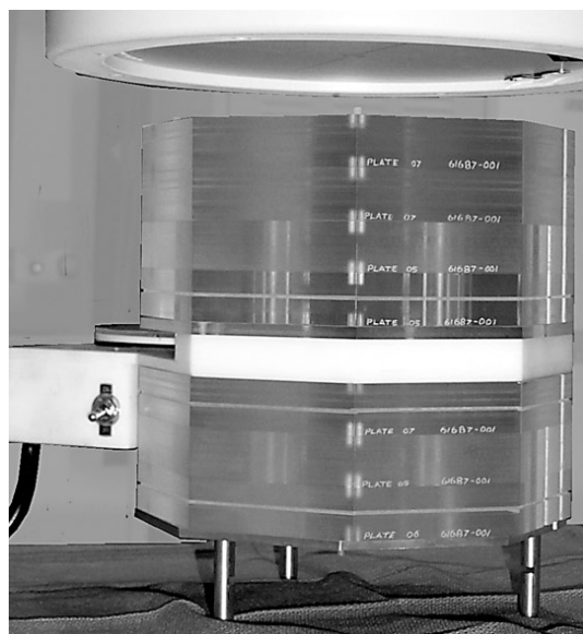
Figure 1. The NEMA Cardiology phantom
