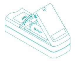
When the low battery symbol is displayed on the LCD or LCD display is dark, replace the old batteries with two new batteries.
