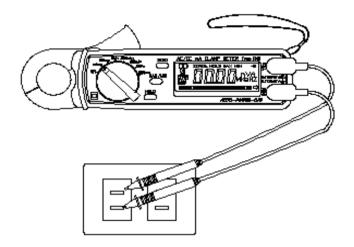
**WARNING**: Maximum input for DC V is 600, and for AC V is 600. Do not attempt to take any voltage measurement that exceeds the limits. Exceeding the limits could cause electric shock and damage to the clamp meter.
