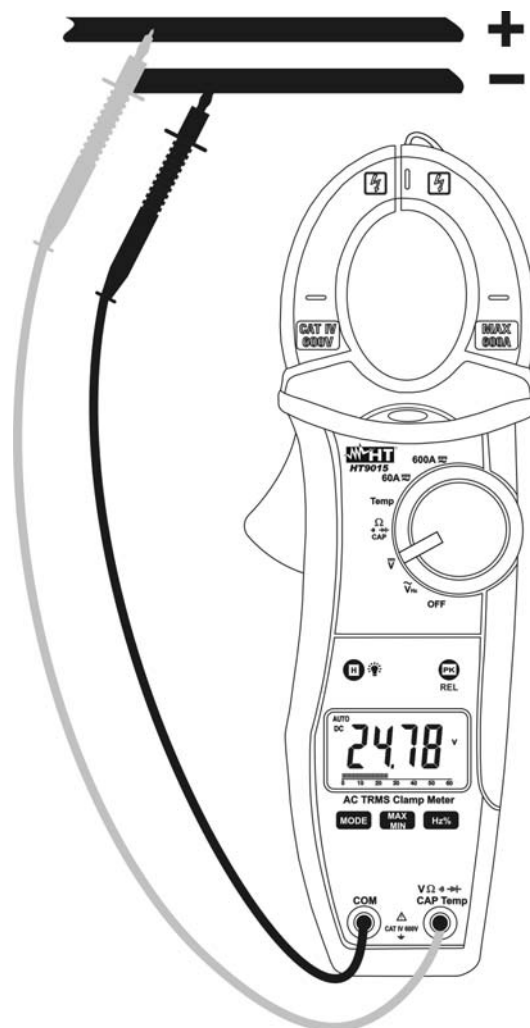
Fig. 8: Taking DC voltage measurements
