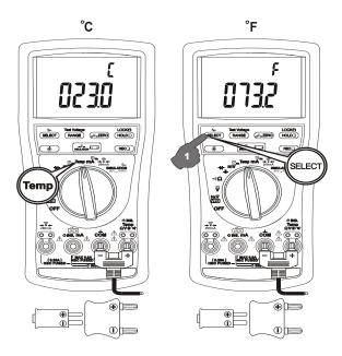
Note: Be sure to insert the banana plug type-K temperature bead probe Bkp60 with correct — polarities. You can also use a plug adapter Bkb32 (Optional purchase) with banana pins to type-K socket to adapt other standard type-K mini plug temperature probes.
