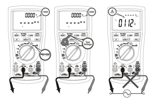
The is active as long as the TEST button is pressed and hold. The TEST buttons on the meter and on the Remote Probe work alike. The Insulation Resistance readings are shown on the primary display.
