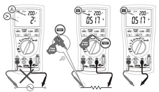
**Lock-Test mode** is recommended for continuous measurements. To apply, press the LOCK button momentarily to display the annunciator **LOCK** before pressing the TEST button momentarily. The LCD will show both **LOCK** & **TEST** to indicate continuous measurement is active. Press again either button momentarily to release the Lock-Test mode.
