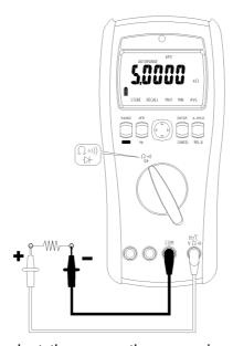
• Press the function button to select the presently measuring function ( $\Omega$  / Continuity Check / Diode Test).
