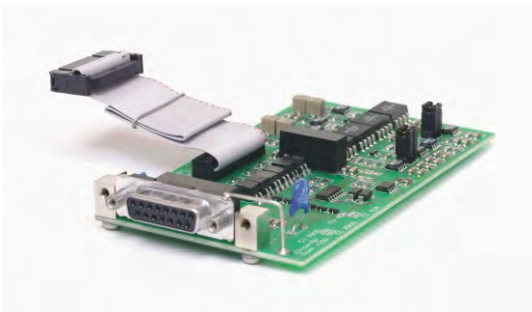
An ISO AMP CARD should be used in case of a non-floating programming source.
