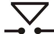
fig. 4 - 10 The Interlock symbol will be visible in the display when the link is interrupted.
