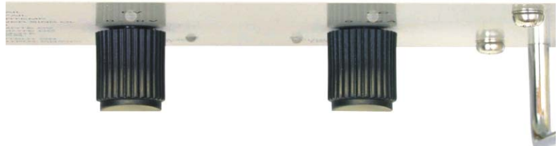
fig. 4 - 17 Meter calibration with 25-turn potentiometers on P596
