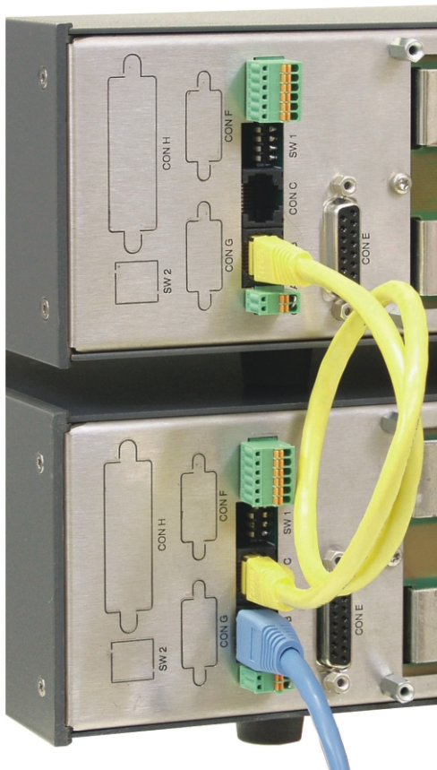
fig 3 - 21 Use standard UTP cables (RJ45) for Master / Slave operation
