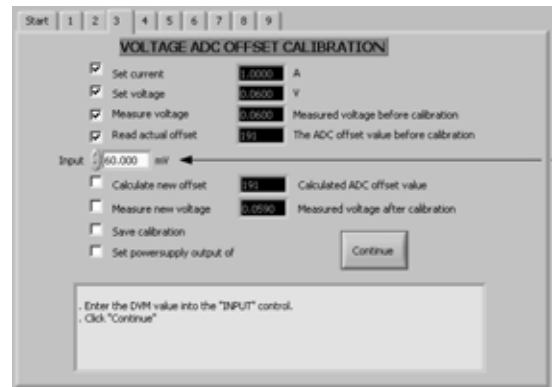
Screen 3: Voltage ADC offset calibration
