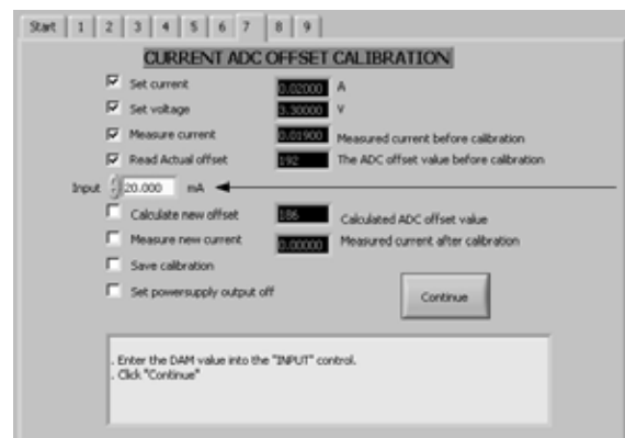
Screen 7: Current ADC offset calibration
