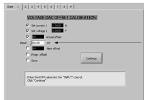
Screen 1: Voltage DAC Offset calibration
