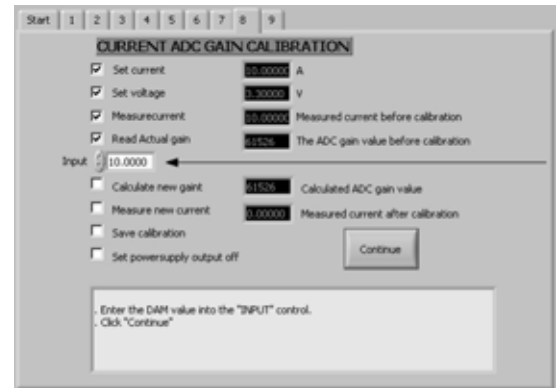
Screen 8: Current ADC gain calibration
