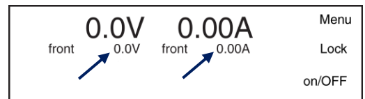
fig 5 - 16 The second line shows the set value for voltage and for source current.
