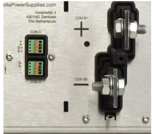
fig 5 - 3 The two DC power terminals CON B1 and B2. Con C and D are the sensing connectors.
