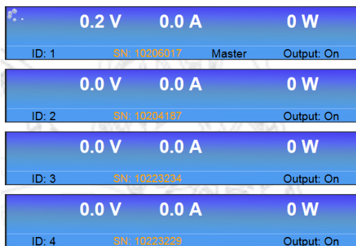
Figure 9.3: Console for Master / Slave monitoring.
