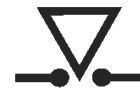
Figure 7.11: The Interlock symbol will be visible in the display when the link is interrupted.
