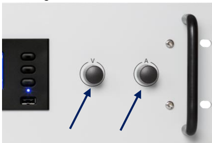
Figure 6.2: Encoders for voltage and current settings
