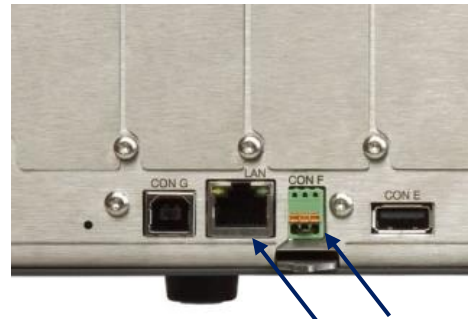
Figure 7.6: The location of the LAN-connector (left) and the Interlock connector (right) at the rear panel
