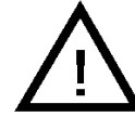
Figure 10.7: If the Internal Error-icon is shown on the display, the DC-power output of the unit will shut down.
