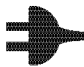
Figure 10.5: If the ACF-icon is shown on the display, the unit has not enough AC input power and the DC power terminals are shut down.
