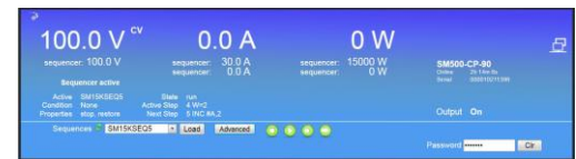
fig 7 - 2 Sequencer console for selecting and controlling sequences.
