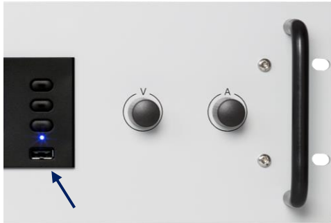
Figure 7.7: The location of the front USB-connector.
