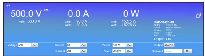
fig 3 - 4 - The front console of the web interface for setting of the output and monitoring various parameters.
