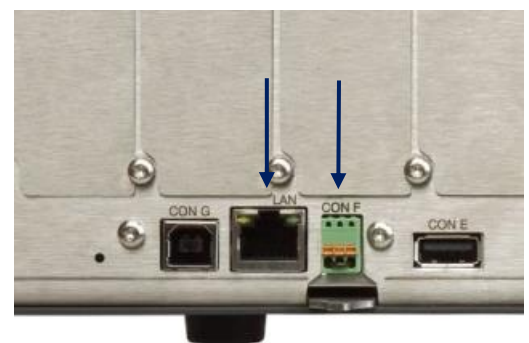
fig 5 - 6 The location of the LAN-connector (left) and the Interlock connector (right) at the rear panel.
