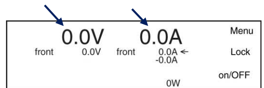
fig 5 - 15 The first line in the display shows the actual output value for voltage and current.
