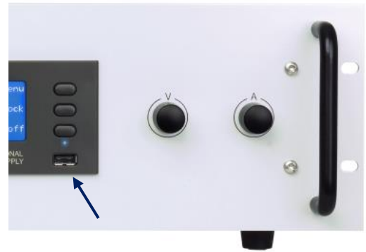
fig 5 - 7 The location of the front USB-connector.
