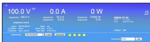
Figure 9.2: Sequencer console for selecting and controlling sequences.
