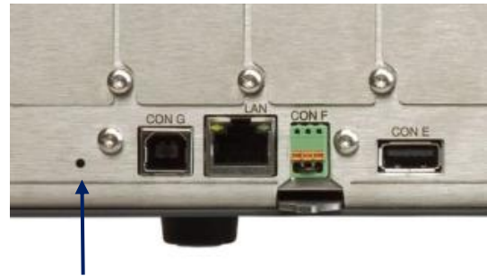
Figure 10.8: Location of the reset button.
