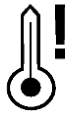
Figure 10.4: If the OT-icon is shown on the display, the unit has run hot and the DC power terminals are shut down.
