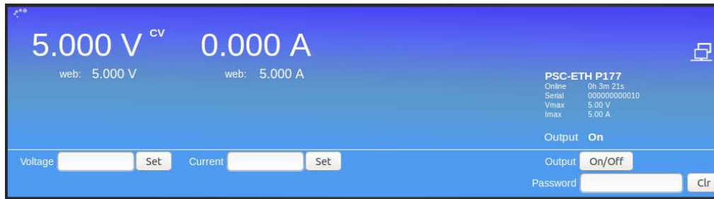
Fig. 4 - 2 - Front console for setting of the output and monitoring various parameters.
